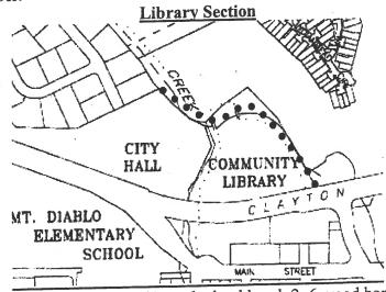
Trail tread - ½ x crushed granite - 6x72' crushed gold rock 2x6 wood border on one side - 8 x 440' - ½ x crushed granite - Level grade - Level cross grade.
