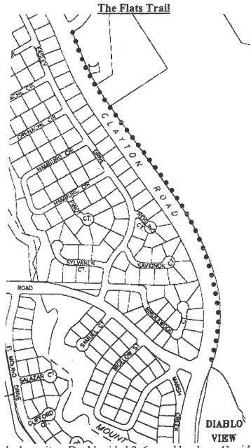
Trail tread - ½ x crushed granite - Double sided 2x6 wood border - 4' wide x 2,787' long - Level grade - Sloped cross grade.
