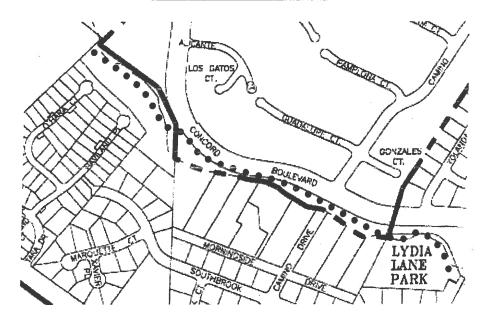
Trail tread - Asphalt base (2 bridge crossings) – 10' x 515', 6'x 62' smooth surface / 6'x 2,169' chip seal surface – Level grade – Level cross grade.
